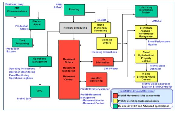
Experion Blend Controller is a key component of Honeywell's Profit® Blending Suite and integrates with other Honeywell applications
