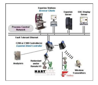
Sample EBC Architecture for Experion Controller-based Systems
