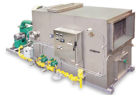
Figure 9: An indirect air heater, which combines an ultra-low NOx burner with a sinusoidal-plate heat exchanger can provide low emissions and effective process air heating.
