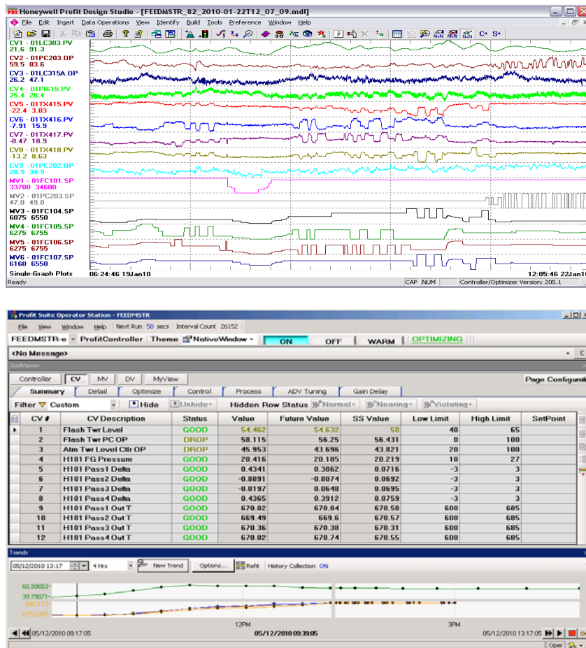
Figure 2. Profit Stepper R320 is a powerful tool designed for automated data collection and step testing.
