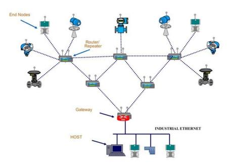
Figure 2. Honeywell's wireless mesh network architecture utilizes externally powered multi-nodes scattered throughout the coverage area.
